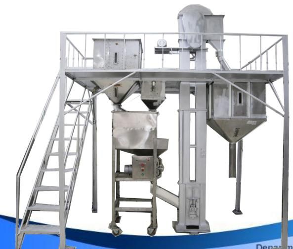
THE FABRICATED **BLENDING** MACHINE HAS AN **ACCEPTABLE FLOW RATE CAPACITY OF 30KG/MIN, WITH HIGH PERCENT** WHOLE GRAIN **RETENTION OF** 95.1%
